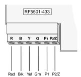
**NOTE:**  $P_1$  and  $P_2$  are open collector programmable outputs. Refer to the control panel manual for proper hook-up diagram.  $P_2$  is also the zone input terminal when programmed (see section [90]). DEOL is supported by this keypad.
